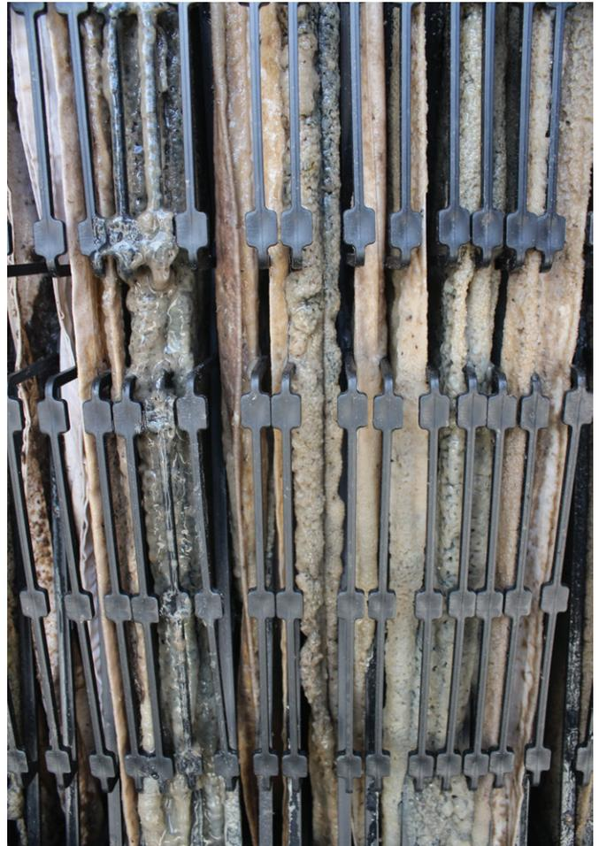
Suspended biomass vertically supported and surrounded by oxygen - a key feature of the BioGill technology.
